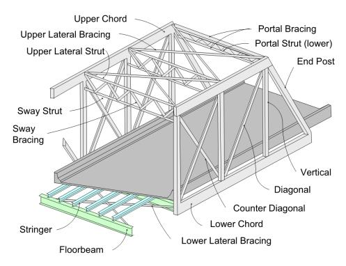
Figure 4 Typical Truss Components [10]
