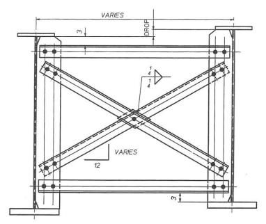
Figure 5 Detail sketch of a typical Knocked-Down cross-frame
