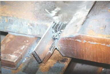
Figure 7 Photograph showing a run-off tab
