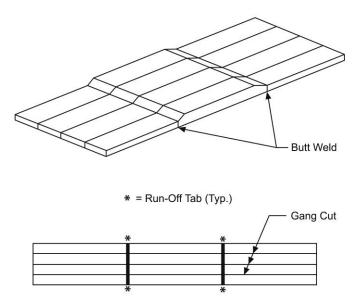
Figure 6 Sketches showing the slabbing and stripping process
