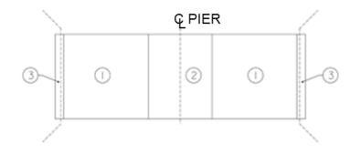
Figure 23 Sample deck placement sequence
