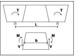
Figure 15: Freebody diagrams for calculating diaphragm forces.
