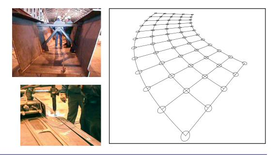
In a grid analysis, a two-dimensional grid is used to define the overall geometry, with line elements used to model the girders and diaphragms... complicated without additional computational aids. More effective methods to consider the interaction of the girders are grid analysis and Three-Dimensional Finite Element Analysis (3-D FEA).
