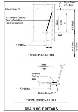
Figure 22: Suggested details for drain holes in tub girder bottom flanges.
