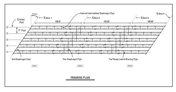
staggered, right (non-skewed) pier diaphragms to simplify detailing and erection. At the end diaphragms, there was not much choice but to detail the diaphragms on the 34-degree skew; the designers consulted a steel detailing shop and a local fabricator during the design process to solicit input on preferred details for the skewed end diaphragms.
