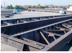
Figure 19: Cost versus benefit: Full shop fitup was required on this tub girder project to help ensure erection would go smoothly. Requiring full bridge assembly in the shop may avoid some fit-up problems in the field, but can be quite costly. Designers are advised to explore all consequences of their decisions.
