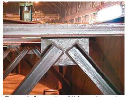
Figure 10: Connection of K-frame diagonals to top chord. Tub girders have many parts and pieces; try to keep the details simple with clean load paths
